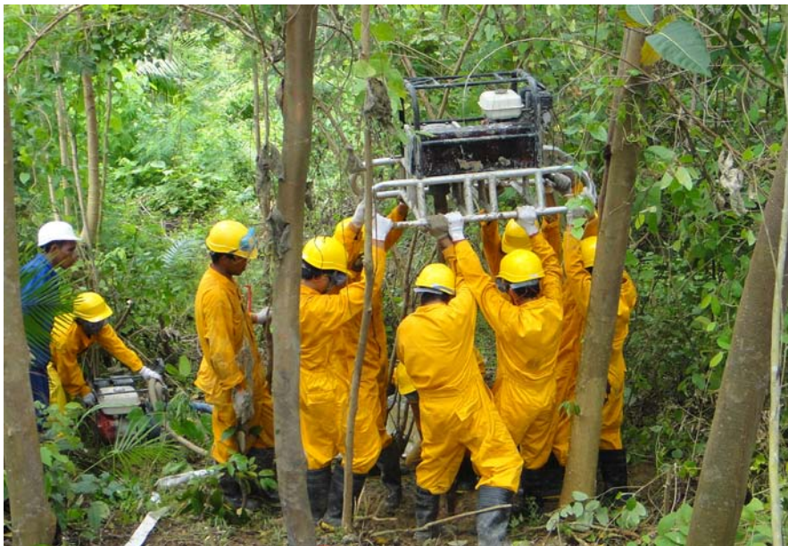
Seismic contractor, BGP's crew auger drilling seismic shot holes, onshore Leyte
