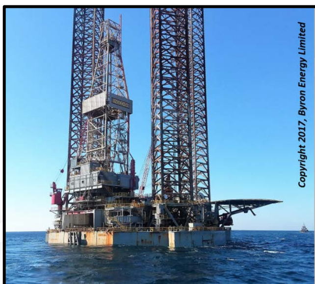
The Ensco 68 independent leg jack up drilling rig under tow on 26 November 2017 in the Gulf of Mexico
